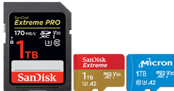
Figure 2.7. Memory card examples with a capacity of 1 TB (Western Digital Corporation, 2016) (Western Digital Corporation, 2019) (Micron Technology, 2019)
