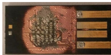
Figure 4.5. USB with no SMD visible
