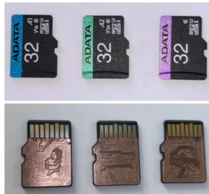
Figure 4.10. Pinouts of memory cards of the same brand and capacity
