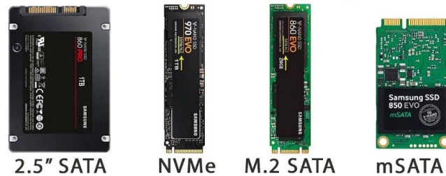
Figure 2.9. SSD interface examples (How-FixIT, 2019)
