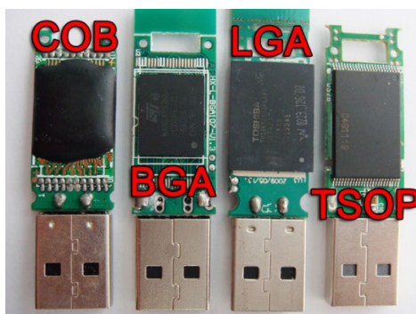
Figure 2.4. Connection types of NAND memory chips to the printed circuit board (Thomas, 2013)
