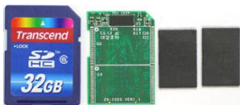
Figure 4.2. Memory card with SMD showing
