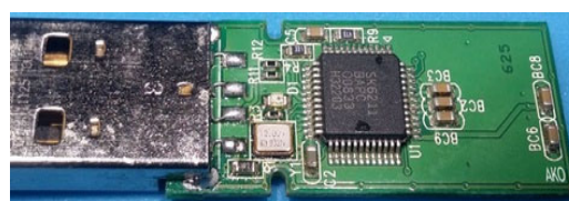
Figure 4.3. USB with SMD showing
